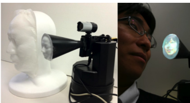
Fig. 20 On the right: Comparison with a real-size face shaped screen and downsized the face-shaped screen at 1/14. On the left: Image of mounting around the shoulder.
