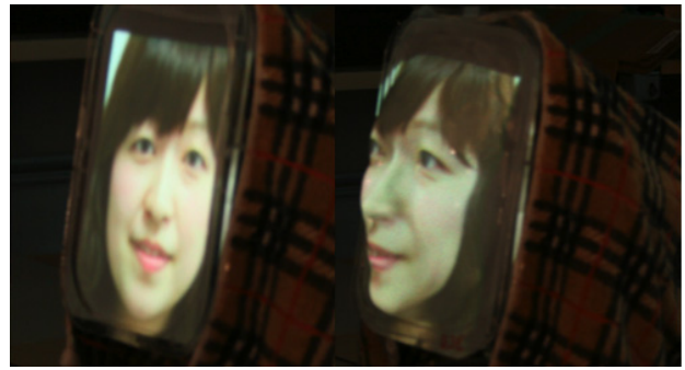
Fig. 23 Comparison of screens - The same image is projected on 2 kinds of screen. The left is a flat screen, and the right is face-shaped one. The each direction of eye gaze looks different.
