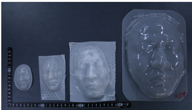
Fig. 19 Comparison of the size: On the left is 1/14 scale face-shaped screen. On the right is the real size face-shaped screen.
