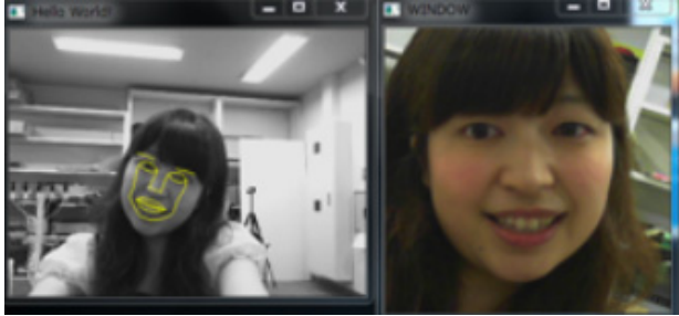
Fig. 6 Image Processing - Screenshot of facial recognition. In the image on the left, the state of head inclined has been adjusted, resulting in the right texture image. The image is inverted for projection.
