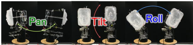
Fig. 5 3DOF - Pan-shaking the head from side to side, Tilt-nodding up and down, Roll-inclining the head from side to side.
