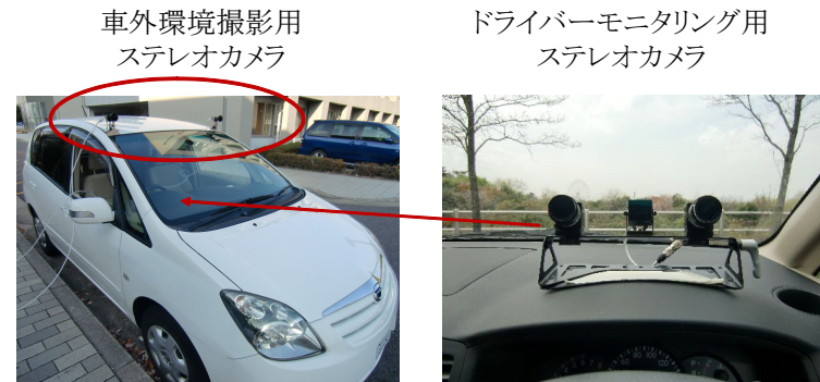
図1 各ステレオカメラの配置の様子 Fig. 1 Appearance of the installation of both stereo cameras
