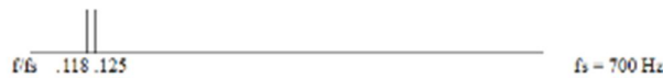
Figure 5 Difference in digital frequency between 82.4 Hz and 87.3 Hz if the sampling frequency is 700 Hz is .125 - .118 = .007
