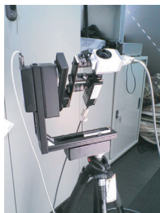
Fig. 6 Panoramic multispectral imaging system
