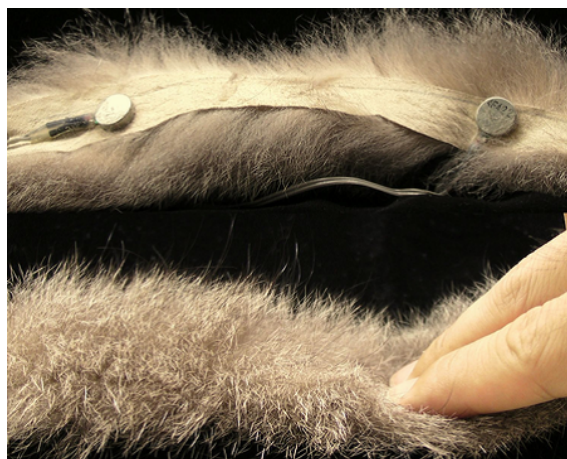
図1 天然毛皮と振動モータの貼付位置 Fig.1 Natural Fur and the Position of Vibration motors.
