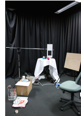
図 2 The environment where we asked the artists to paint. The room is covered with black curtains to avoid interreflection from the walls. The painters are requested to paint the scene visible inside the white window frame, so that every artist has similar views.
