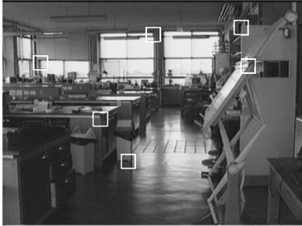
Fig 4: Typical features used in a visual mapping system: an image interest operator locates patches with high intensity gradients in both the x and y directions. These typically correspond to the corners of scene objects and are well localised in space, though reflections or depth discontinuities can also throw up unsuitable candidates: in SLAM, these can be rejected over time since they do not behave as stationary landmarks when observed from new viewpoints.
