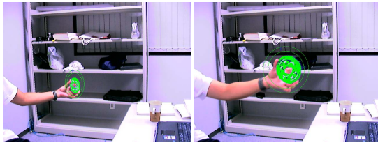
(a) Tracking a CD-ROM having a hole and high-light patterns in translation, rotation in depth and zoom
