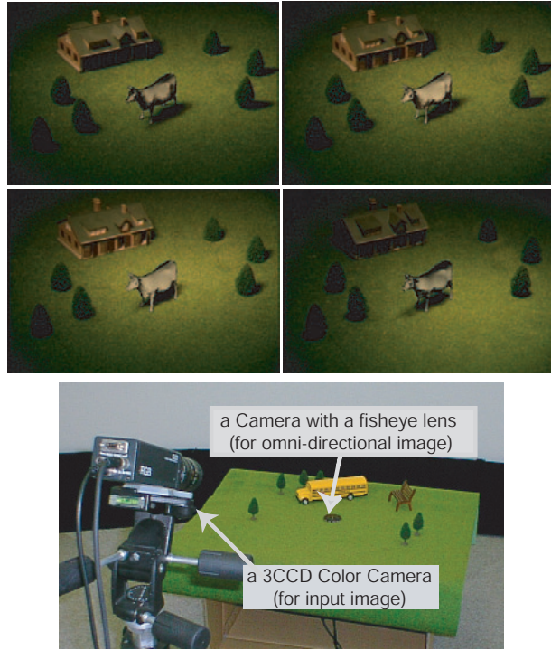
Fig 3: Image acquisition system and synthesized images by our method: a color camera with a fish-eye lens is used for capturing illumination of the scene.
