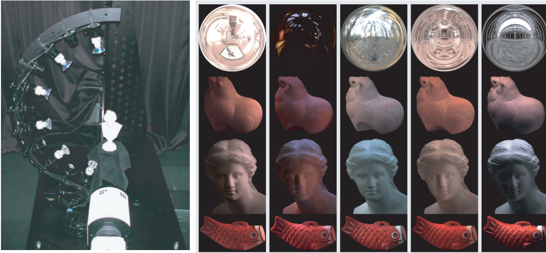
Fig. 7: Hardware set-up and synthesized images of objects under natural illumination. The first row shows illumination maps. The second, third and fourth rows show synthesized appearance of objects under the corresponding illumination map.
