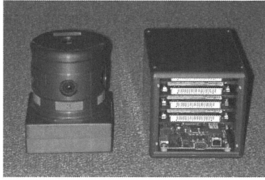
Fig. 4: Omni-directional multi-camera system: Ladybug.
