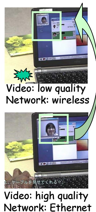
Figure 12. The system controls video quality according to network bandwidth. When a user unplugs the Ethernet cable from the PC, the video phone session is handed over to a wireless connection, and, at the same time, the quality of video image becomes lower.
