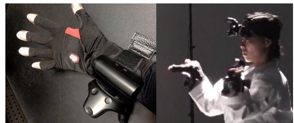
Fig.1 Hi5 VR glove (left) and karate performer with VIVE trackers on head and hands.
