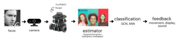
Fig. 1 Our pipeline for facial expression-based emotion recognition and application to the robot.
