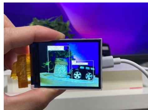
Figure 1 Example of object detection by edge device.
