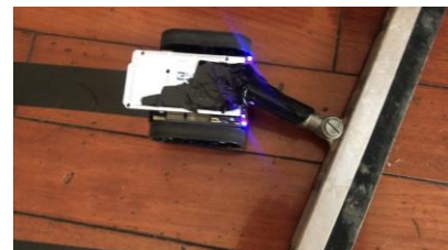
Fig. 2 Broom installed behind the Zumo robot.
