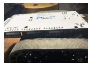
Fig. 3 Arduino board is connecting with Zumo robot. Arduino is an open-source electronics platform [6]. The Arduino code uses in all process of controlling the robot.
