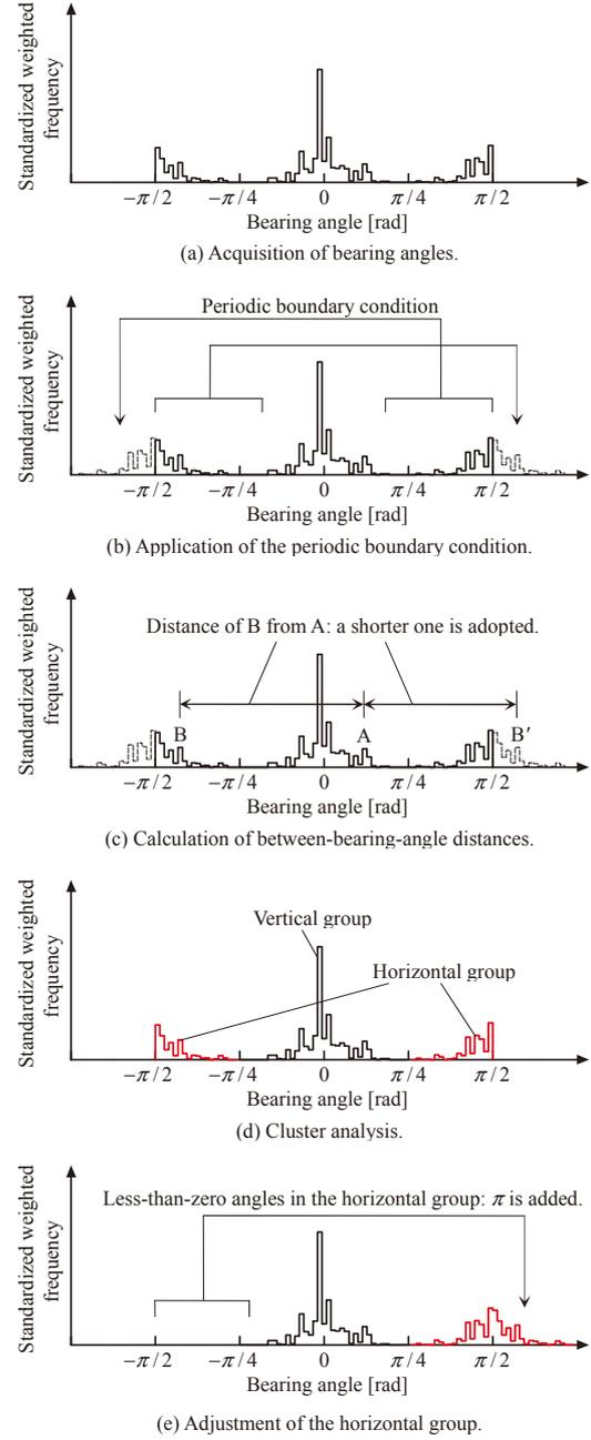
**Fig. 5** Grouping of the bearing angles of line elements.
