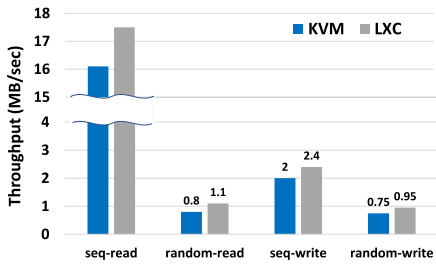
Fig. 4 Disk I/O throughput in KVM and LXC in consolidation case when two I/O workloads are collocated together. LXC outperform KVM in all workloads.
