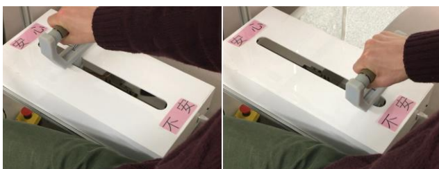
図 8 安心感入力装置 Figure 8 An input device for subjective sense of comfort.
