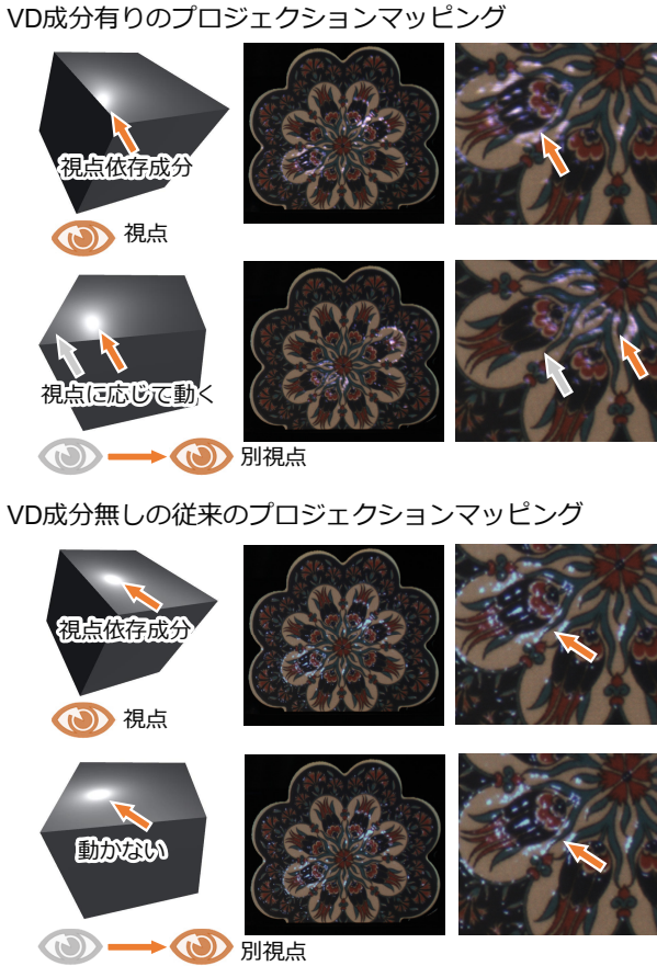
図1 VD成分有り, 無し of 質感再現 Fig.1 material reproduction with and without VD components
