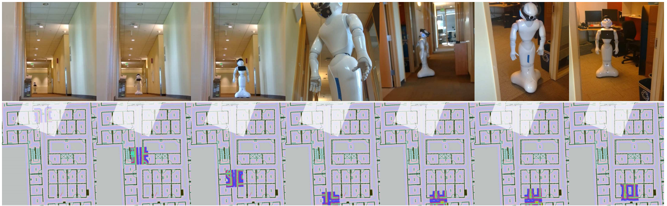
図 7 Navigation with our system using external SLAM device. Lower sequence is floor map in GUI. First, Pepper walks long corridor and then turn at the corner. Finally, Pepper enters a room and reaches to the destination.
