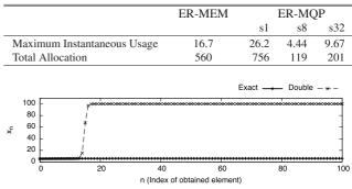
Fig. 7 Values of  $x_n$  (n = 0, ..., 100) of Muller's sequence. The x-axis corresponds to the index n of  $x_n$ . Lines show the results of double-precision arithmetic and exact values.
