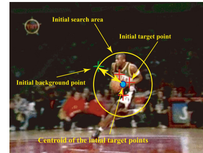
Fig. 16 Initialization for multi-color object tracking.
