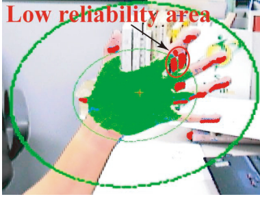
Fig. 4 Outliers are detected and painted with red by our RK-means algorithm.
