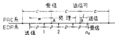
図 12 EDP 系と PRC 系の情報伝達手順 Fig. 12 Data communication procedure between EDP and PRC system.
