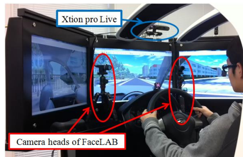
Fig. 2 Experimental system for measuring driver's behaviors.
