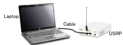
Fig. 6 USRP and laptop connected via an ethernet cable in each measurement set.
