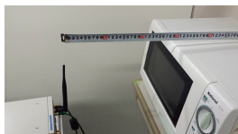
Fig. 5 USRP deployed 0.3 m away from the front door of microwave oven.
