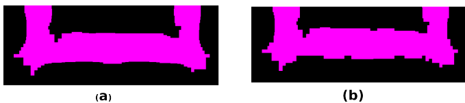
Fig. 12: Portion of Benchmark 5 Mask: (a) Before Post OPC. (b) After Post OPC.
