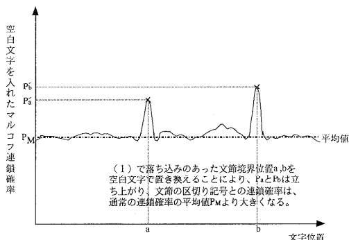
(2) 文節境界の認定法 Method to estimate the boundary of bunsetsu using space symbol.
