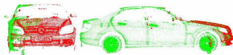
図 16 Results of registration of point clouds from directions 0-2 by a proposed method.
