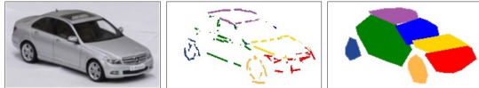
図 12 The left is a picture of the target object. The middle is an image of color-coded parts with an estimated active curves from the image on the left. The right is an image that the inside area embedded from the active curves in the image in the middle.
