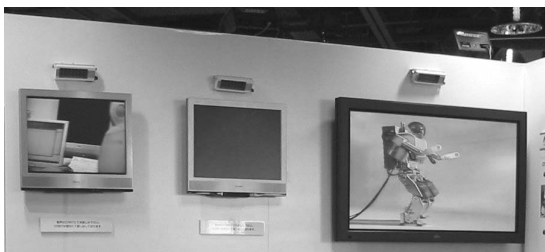
図 19 LED24 個タイプの CoBIT 用光源 Fig. 19 Infrared LED emitters for CoBIT.
