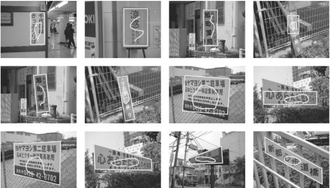
図 3 各探索法による看板抽出結果（上段は長方形探索，中段は回転探索，下段は 4 辺探索） Fig. 3 Results of the signboard extraction by each region search method (upper: rectangular search, middle: rotational search, lower: four-side search).
