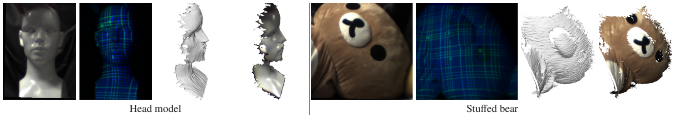
Fig. 15 3D reconstruction with texture mapping of a head model (left) and a stuffed bear (right). The figures are the image of visible light, the IR image, the shape without texture, and the textured 3D shape, respectively.
