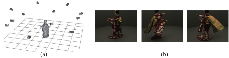
Fig. 22 Camera arrangement and input images. (a) 12 XGA cameras. (b) Example frames taken by one of 12 cameras.
