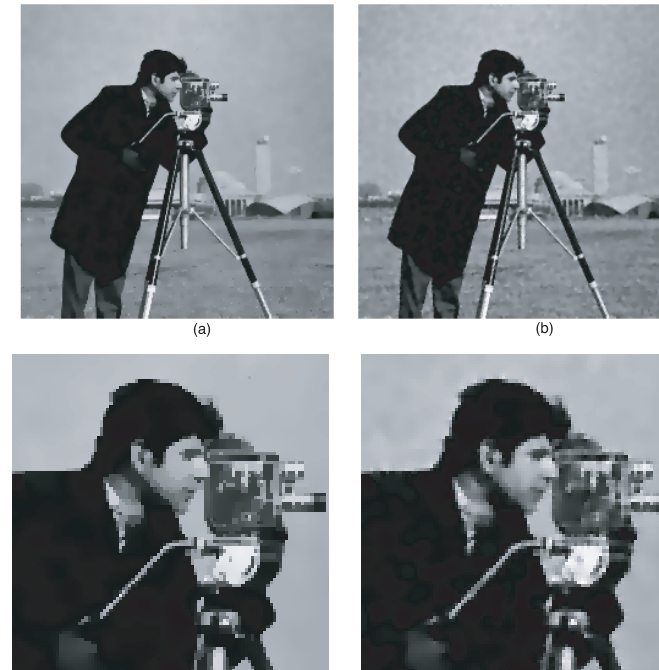
Fig. 7 Comparing the perceptual quality of the results obtained by proposed and Perona-Malik filters for noisy image of Cameraman shown in Fig. 4. The images labeled (a) is the result of the Perona-Malik filter and (b) is the result obtained by the proposed filter. A magnified region of each denoised image is shown in the second row.
