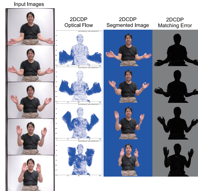
Fig. 15 Pixel tracking using 2DCDP(2): The result of pixel tracking using arbitrary shapes. 2DCDP was able to track object deformation.
