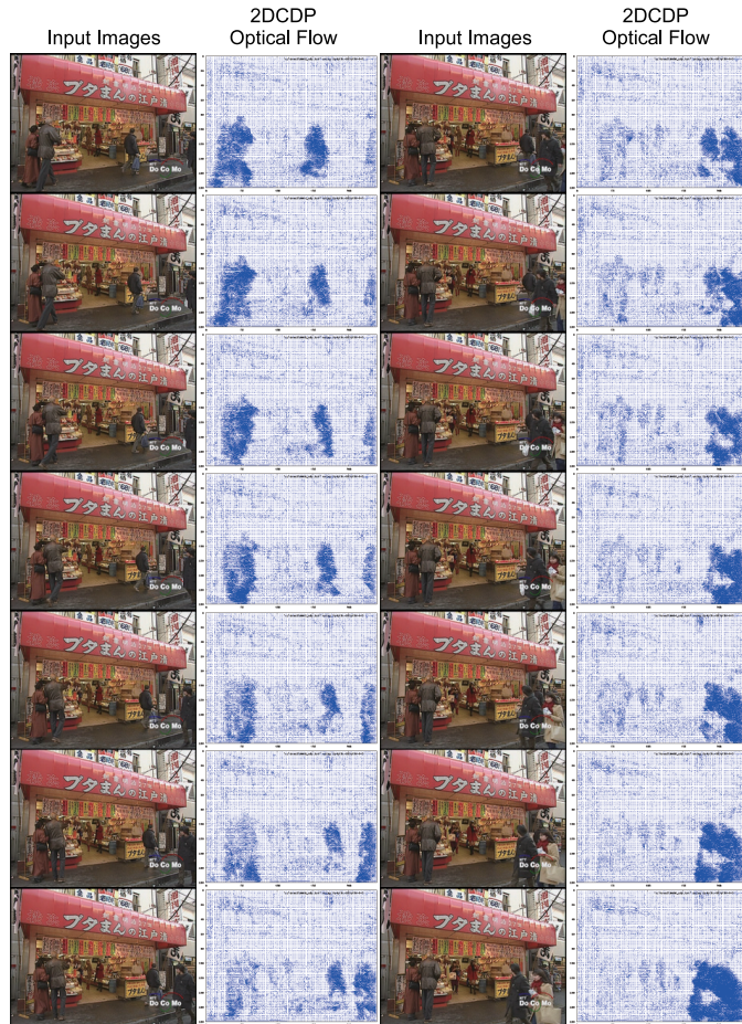
Fig. 14 Pixel tracking using 2DCDP(1): The second and fourth columns show the result of tracking multiple objects from the first and third columns. Our proposed method extracts precise pixel flows caused by the motion of multiple objects. Occlusion and emerging new objects in a stream of time-varying images make up a small part of the pixel flow image.
