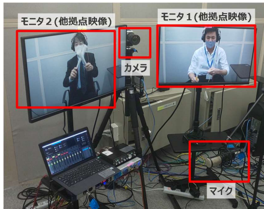
図 5 各ユーザ拠点 (防音室) の機器配備の様子 Figure 5 Deployment of equipment at each user site.
