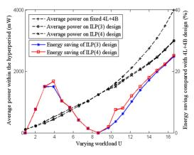
Fig. 7 The effectiveness of core type design: the tendency of energy saving with varying workload.
