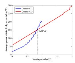
Fig. 6 The energy relation of big and little cores with varying workload.
