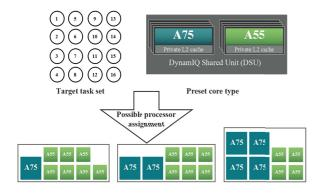
Fig. 1 Flexible core number design announced with DynamIQ technology.
