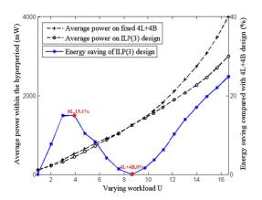
Fig. 5 The effectiveness of core number design: the tendency of energy saving with varying workload.
