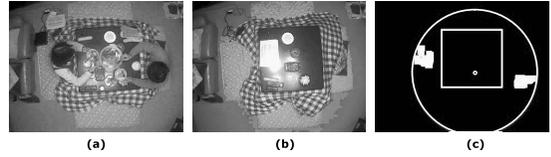
**Fig. 7** Visual tracking results. (a) shows an input image. (b) shows updated background image. (c) shows occupants' location. White areas show occupant's location. White rectangle shows the table area. White circle shows circle enclosing occupants' mass. Note that the table area was manually extracted.
