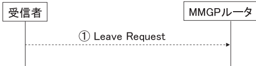
図 5 非トークンメンバの離脱 (MMGP Leave) 手続き Fig. 5 Leave procedure for the non-token member (MMGP Leave).
