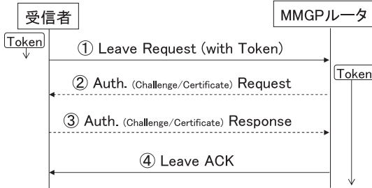
図 6 トークンメンバの離脱 (MMGP Leave) 手続き Fig. 6 Leave procedure for the token member (MMGP Leave).
