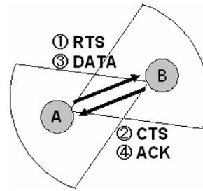
Fig. 5 Data transmission using DVCS.
