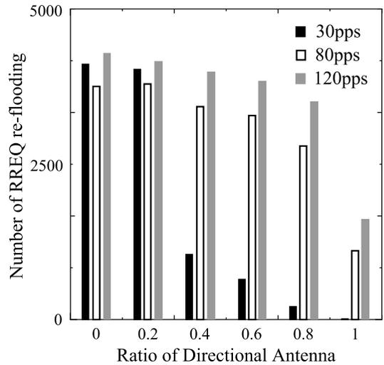
Fig. 8 RREQ re-flooding performance ( $R = 1.8$ ).
