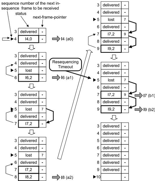
Fig. 7 An example of resequencing procedures including a timeout.
