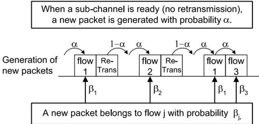
Fig. 9 A packet generation model of multiple real-time flows.
