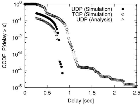
**Fig. 11** Complementary Cumulative Distribution Function (CCDF) of real-time (UDP) and non-real-time (TCP) packet delays by MQ-PFRS ARQ, where the bit error rate  $B_{ERR}$  is  $10^{-6}$ .
