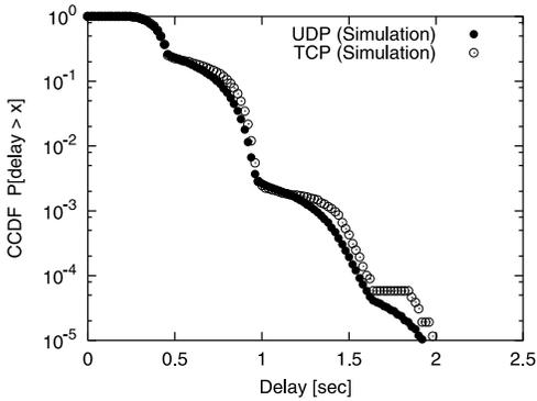
**Fig. 15** Complementary Cumulative Distribution Function (CCDF) of real-time (UDP) and non-real-time (TCP) packet delays by PFRS ARQ, where the bit error rate  $B_{ERR}$  is  $10^{-6}$ .
