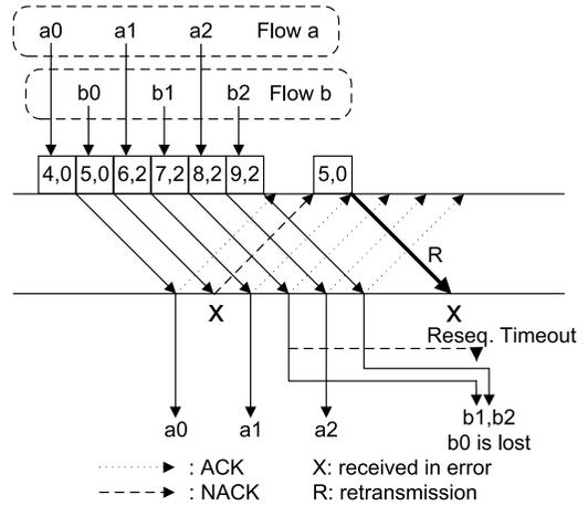
Fig. 4 An example sequence of MQ-PFRS ARQ.
