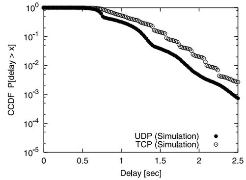
**Fig. 14** Complementary Cumulative Distribution Function (CCDF) of real-time (UDP) and non-real-time (TCP) packet delays by conventional SR ARQ with priority queues, where the bit error rate  $B_{ERR}$  is  $10^{-5}$ .
