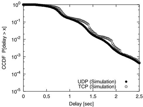
**Fig. 16** Complementary Cumulative Distribution Function (CCDF) of real-time (UDP) and non-real-time (TCP) packet delays by PFRS ARQ, where the bit error rate  $B_{ERR}$  is  $10^{-5}$ .
