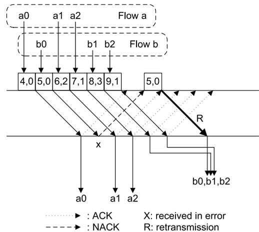
Fig. 3 An example sequence of PFRS ARQ.
