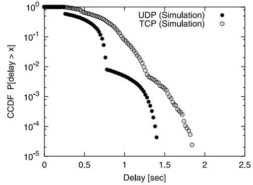
**Fig. 13** Complementary Cumulative Distribution Function (CCDF) of real-time (UDP) and non-real-time (TCP) packet delays by conventional SR ARQ with priority queues, where the bit error rate  $B_{ERR}$  is  $10^{-6}$ .
