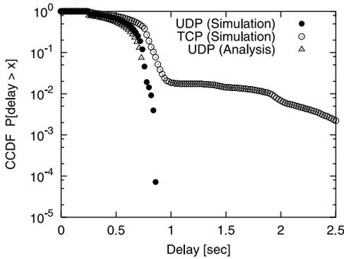
**Fig. 12** Complementary Cumulative Distribution Function (CCDF) of real-time (UDP) and non-real-time (TCP) packet delays by MQ-PFRS ARQ, where the bit error rate  $B_{ERR}$  is  $10^{-5}$ .
