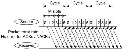
Fig. 8 An SR ARQ model employed in the analysis.
