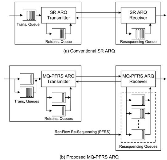
Fig. 1 Construction of queues in conventional ARQ and in MQ-PFRS ARQ.
