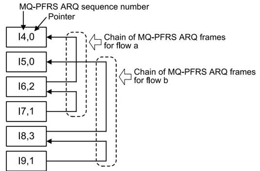
Fig. 6 Identification of frames belonging to the same flow by the pointer.
