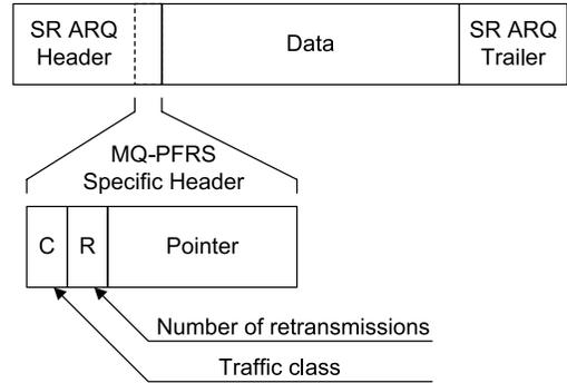
Fig. 5 MQ-PFRS ARQ specific frame header information.
