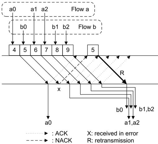
Fig. 2 An example sequence of the conventional SR ARQ.
