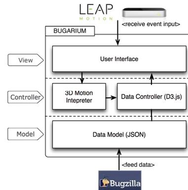
Fig.1 The structure of Bugarium
