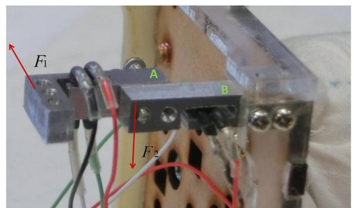
Fig. 4 Force Sensor Equipment
