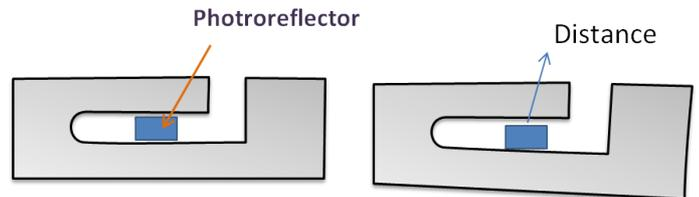
Fig. 3 Force Sensor Deformation Before and After
