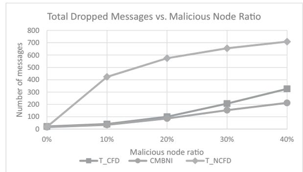
**Fig. 6** Total message drop vs. Malicious node ratio (Sink center).
