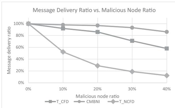
**Fig. 5** Message delivery ratio vs. Malicious node ratio (Sink edge).
