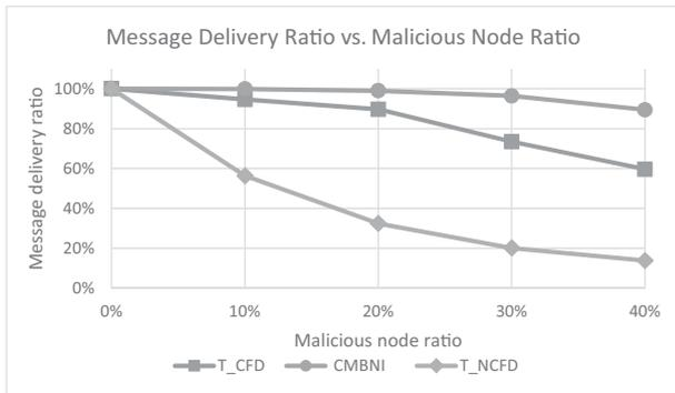
**Fig. 4** Message delivery ratio vs. Malicious node ratio (Sink center).
