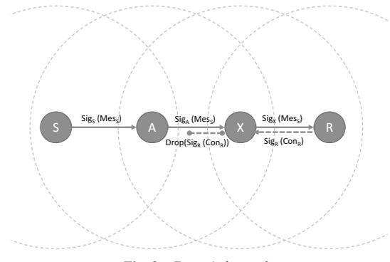
Fig. 2 Drop Ack attack.
