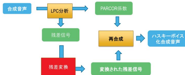
図 2 残差変換法に基づくハスキーボイス化の処理フロー Fig. 2 Processing flow of the husky voice of based on residual conversion method.
