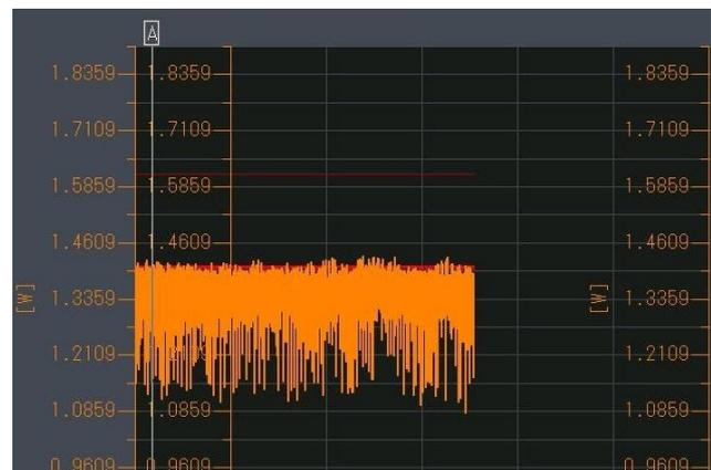
Figure9: Power consumption on RPX using power optimization
