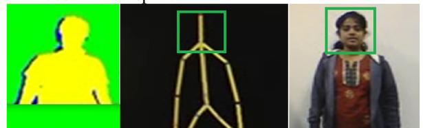
Figure 4. Head Tracking using depth cues from kinect sensor
