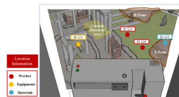
Figure 1. AR user interface in a construction site
