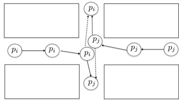
**Fig. 2** Example pseudonym exchange. Two users exchange their pseudonyms  $p_i$  and  $p_j$  at the intersection. The solid lines denote each user's actual path while the dotted lines denote an alternate possible path.
