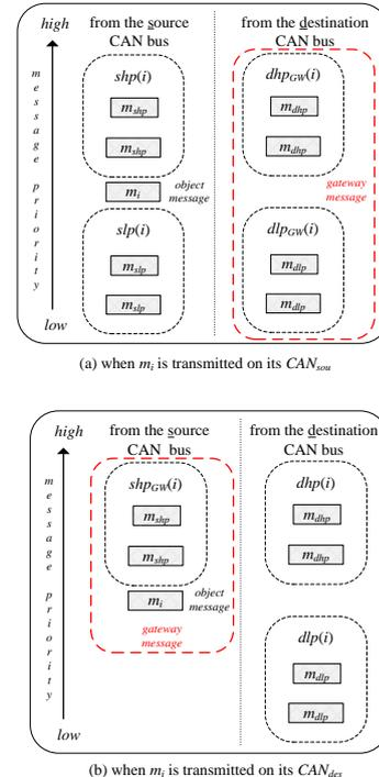
Fig 3: Interference analysis for CAN messages
