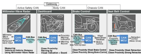
Fig 1: Gateway-based implementation of Collision Detection System [3]
