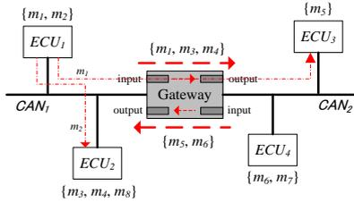
Fig 2: System architecture for automotive electronic system
