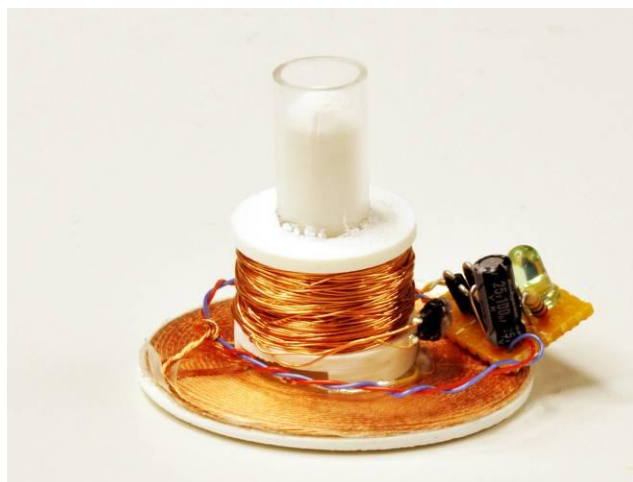
図 13 受電デバイス内部 figure 13 The inside of a receiving electricity device
